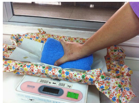
Fig. 5 Test of compression force on electronic baby weighing scale
